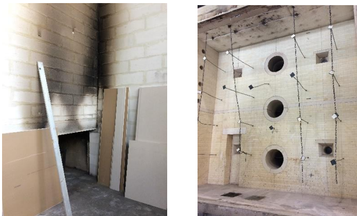
Test rig for analysis of "reaction to fire" behaviour
